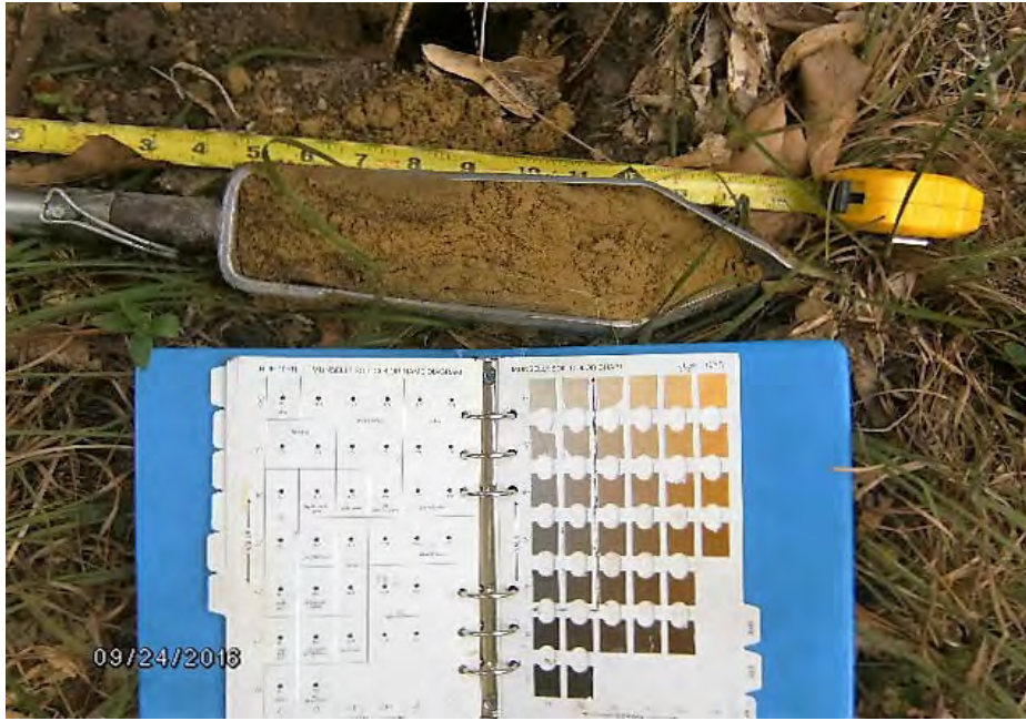
Plot Up - 39 Soil profile showing bright soil chroma with no hydric indicators.
