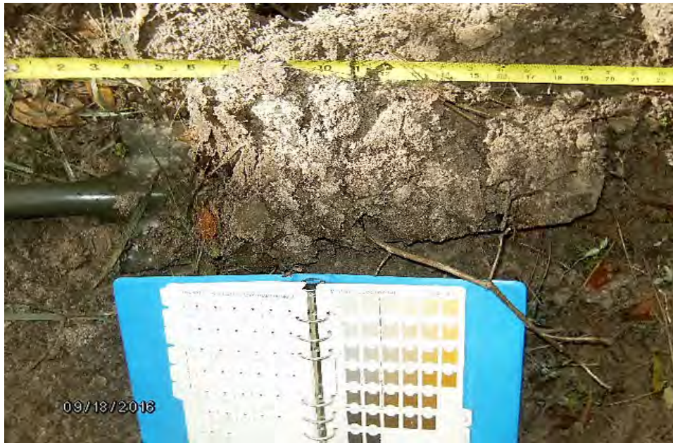
Plot Wet - 15 Soil profile illustrating mostly matrix depletions and low chroma conditions.
