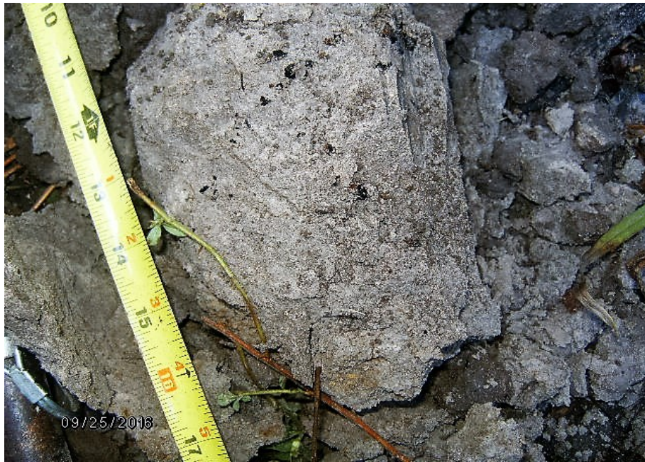
Plot Wet - 40 Lower chroma soils showing evidence of depleted matrix within bottom land drainage area near the Upland plot.
