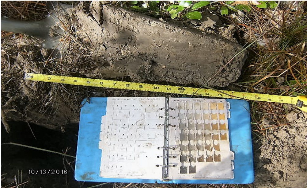
Plot Up - 14 - Soil profile at Up-14 showing low to medium soil chroma 2 and 3.
