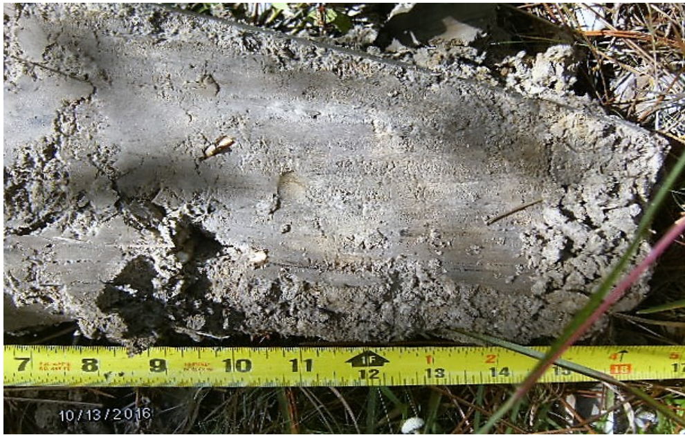
Plot Wet - 14 - Soil profile illustrating increase in Redox concentrations with depletions.
