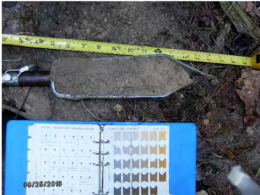
Plot Wet - 52 Soil profile illustrating slightly lower chroma soil material with small signs of Redox concentrations.
