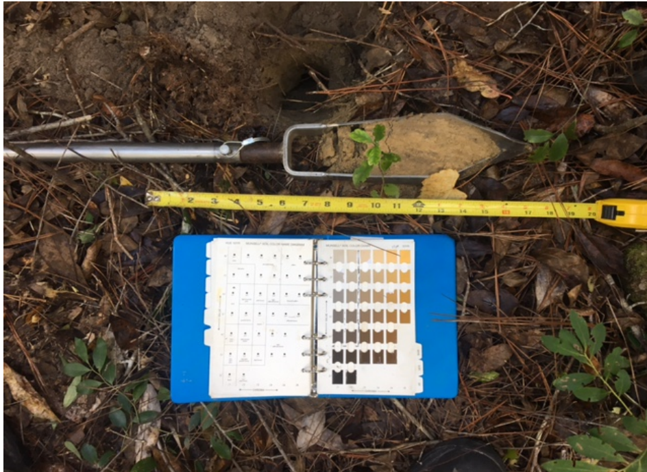
Plot Up - 23 Soil profile illustrating generally bright soil chroma with no hydric indicators.
