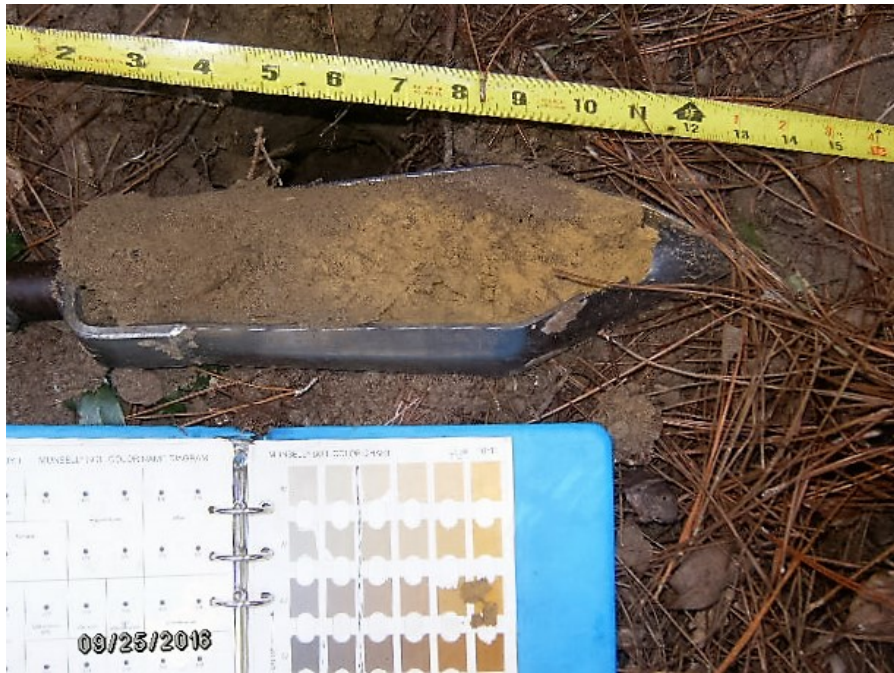
Plot Up - 52 Soil profile illustrating higher chroma, loamy silt/sand within Upland area near the northeast corner of the AOI.
