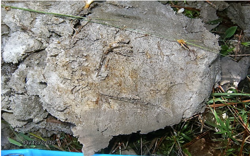
Plot Wet - 11 - Depleted matrix and sandy redox (hydric indicators) in wetland plot.
