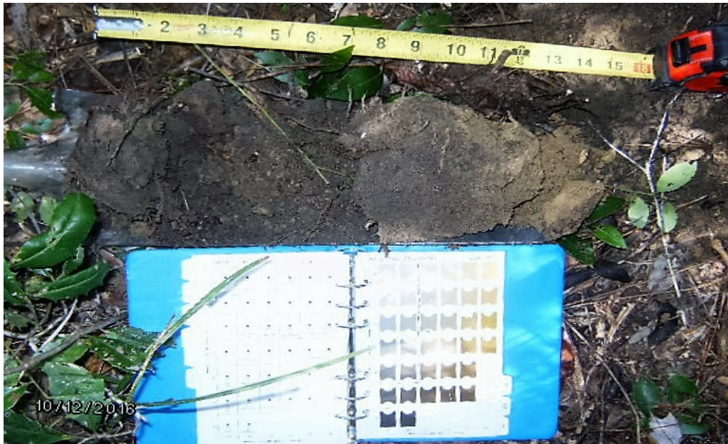
Plot Up - 11 - View of soil transitioning to brighter chroma in upland within Western AOI.
