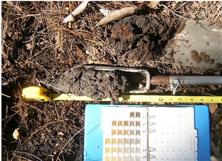
Plot Wet - 33 Low chroma soils with evidence of Redox concentrations.
